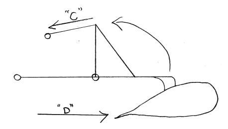
For a given working depth and speed the draught 'D' is proportional to the compression 'C' in the top link.
