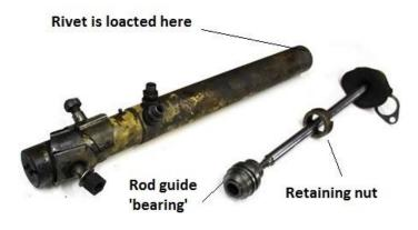
Next simply remove the ram rod guide (this is referred to as the 'bearing' in the Nuffield manuals) along with all seals as shown below. You will need to reuse the following components - circlip, aluminium washer and steel housing seal ring.
