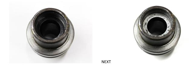
Place in the new O-ring (No 3) next followed by the steel housing seal ring (No 4).
