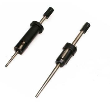
These tools are still available but very expensive; we at Tractor Spare Parts Ltd have redeveloped 37D2599 so it can be fitted without the over rolling tools. It's worth noting these new sleeves can also be used on the 4/98 and 6/98 series of engines. When used on these engines you do not have to fit the loose injector washer 86K1099.
