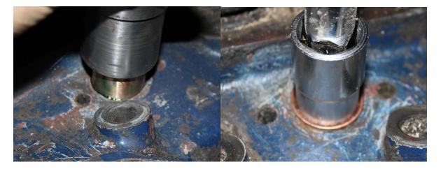
Finally use the back side of a socket and extensions bar to swell the open end sleeve.
