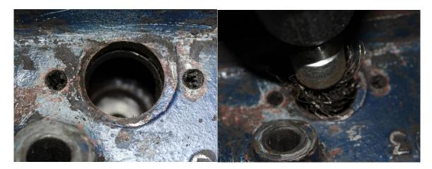
Next check there are no burrs around the edge of the hole, as if burrs are not removed they will damage the side of the injector sleeve as it's fitted. Fit new o-ring 86K906 if required, next apply high strength bearing retainer (Loctite, Bondloc Studlock B270 are the brands we use or an equivalent) around the top the sleeve and in the bore in the cylinder head.
